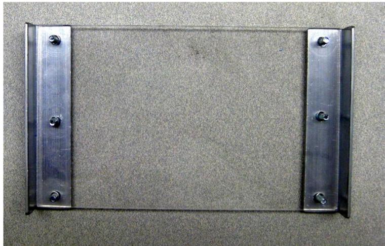
Place the angle aluminum as shown. The piece with the center hole is on one end (the front) and the double piece is on the other. Note the location of the screws on the rear piece. Secure by screwing four 7/8" female-female standoffs onto the 6x32x1/2" bolts on the front section and with two 1 1/4" female-male standoffs on the rear.
