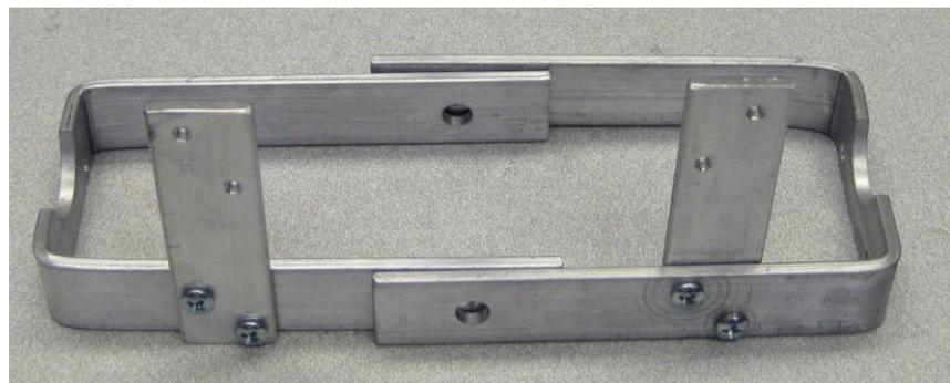
Mount the 3/8" angle aluminum to the tops of the shock towers using 4x40x3/8" bolts and nylon locking nuts.
