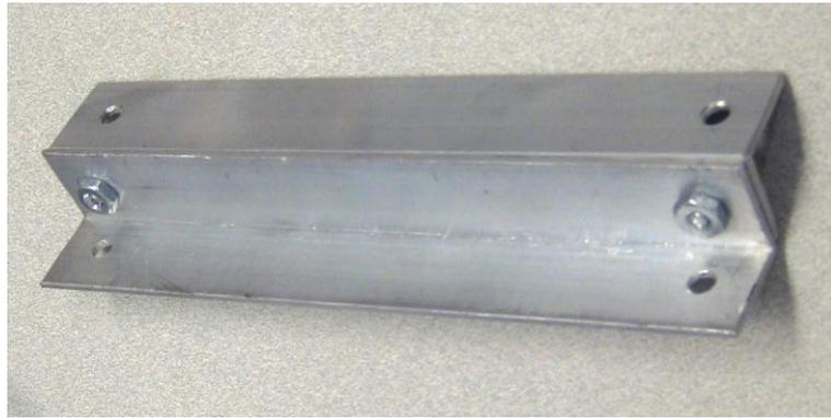
Remove the blue protective film from the Plexiglas. Place 6x32x1/2" bolts through the 3 1/2" angle aluminum and place the Plexiglas over the bolts.
