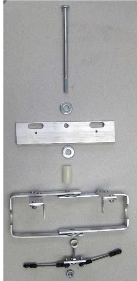
Assemble kingpin parts. Tighten nut so that it is snug but the sway bars still can move freely.
