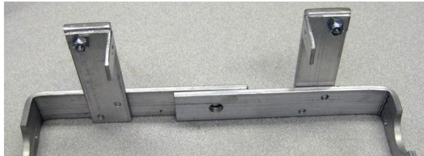
Thread the stabilizer bar ends onto the 4x40 allthread. Screw both ends until 1 1/8" allthread remains visible.
