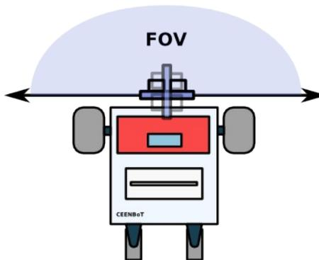
Note that the center position of the 180 degree range is achieved by sending a pulse of 1.5ms every 20ms to the servo. To achieve an angular position of up to 90 degrees to the left or 90 degrees to the right of this center position, you will increase or decrease the pulse width until you achieve your desired sensor position.
