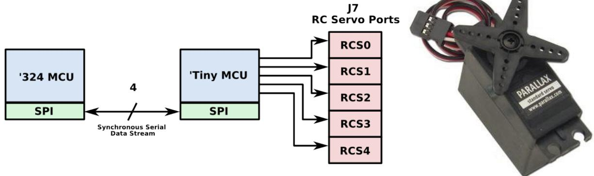
The control structure is similar to that for the IR sensors – they're under the control of the ATtiny. Therefore, to control the servos, *it is necessary* to talk to the 'Tiny. Controlling the servo is fairly straight forward – there are two functions to be aware of from the `TINY` subsystem module in the API. These are:
