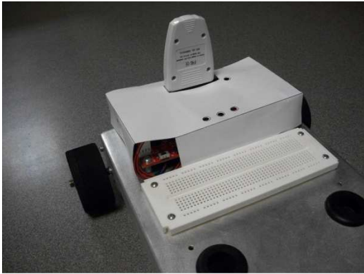
Cardstock prototype design for plastic shell of CEENBoT.
