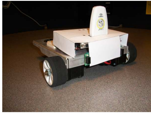
Front view of cardstock prototype design for plastic shell of CEENBoT.
