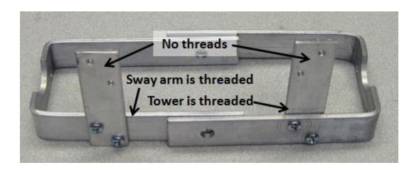
Mount the 3/8" angle aluminum to the tops of the shock towers using 4x40x3/8" screws and nylon lock nuts.
