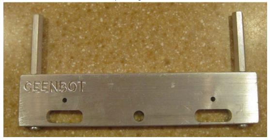
Mount the two Sensor boards on the bumper using the  $4-40 \times 5/8$ " screws and nylon lock nuts. Note that they are mounted on the back side (the side without the CEENBOT engraving) and the red LEDs are on the outside. **Put two fiber washers between the bumper and each board.** This prevents the board from touching the metal bumper and shorting out.
