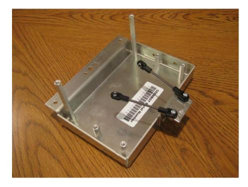
Attach the tray to the Kingpin with the  $\mbox{\em 1}''$  hex nut. Tighten securely.
