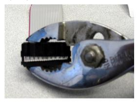
When completed, the plastic of the top part should be against the plastic of the other part.
