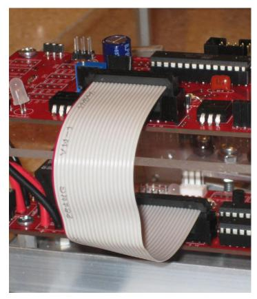
Connect the PlayStation controller card's 20 pin female connector to the 20 pin male connector located on the right side of the Interface card. The
