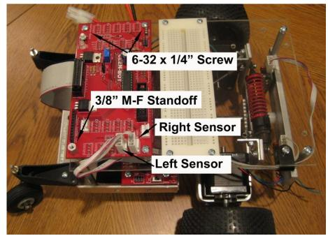
connector SO on the Interface board. Route the wires through the cable holder and the hole in the rear of the Plexiglas.
