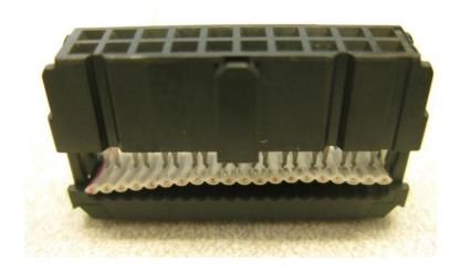
Use pliers to force the connector together. The type of pliers shown works well because they can exert fairly even pressure on the surface. Needle nose pliers usually do not work well.
