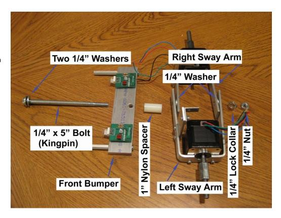
You can use a tapered punch or pencil to align the parts to ease assembly.
