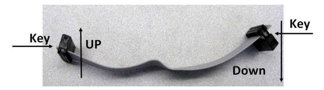
Connect the ribbon cable to the back two connectors on the Interface and Control boards. The plastic key will only allow you to place it one way.
