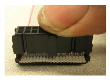
Press on the connector. You will hear two clicks as each end engages. The metal prongs should hold the wires in place.
