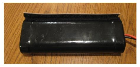
with the exposed adhesive into the open space on the tray behind the Control Board. Remove the battery and the Velcro will separate leaving the hook piece adhered to the tray. Press the hook piece so that it is fully adhered to the tray.
