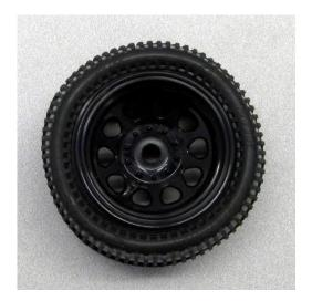
Position the elongated inner bolt on the motor shaft such that it does not touch the frame when the motor turns. The exact position is not important. Attach the wheels to the motors using the hex nut. The molded hex depression in the wheel goes towards the motor. Use a socket wrench to tighten the nut. Do not over tighten or the plastic wheel may crack.
