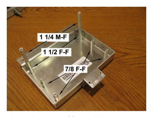
Attach the stabilizers to the tray as shown using 4x40x1/2" screws and locking nylon nuts.
