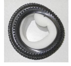
Work the tire over the wheel and adjust so that the tire bead is adjacent to the outer flange of the wheel.
