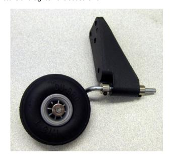
Mount the tail wheels to the tail ledge with  $6-32 \times 1/2$ " screws and nylon lock nuts. Install with the lock nuts on the top. The photo shows them backwards. The larger surface area against the plastic provides more strength and the plastic bracket is not as likely to break on hard landings.
