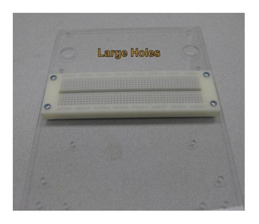
Attach the Plexiglas with  $6 - 32 \times \frac{1}{2}$ " screws on one end and 3/8" M-F standoffs on the other. Note position of large holes.
