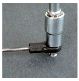
Thread the stabilizer bar ends onto the 4x40 allthread. Screw both ends until 1 1/4" allthread remains visible. You may need to cut about ¼" from the allthread to get this distance. The lab instructor has a cutting cutting tool to do this.
